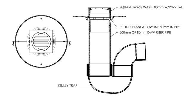
From the inventor of the Leak Control (Puddle) Flange; the Art International Shower Waste Kit combines the confidence of high quality fittings and the convenience of an easy to install kit. The Puddle Flange integrates with the waterproofing membrane, whilst still allowing sub tile water to escape into the drainage.
